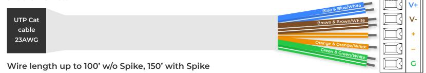
The majority of standard Category cable utilizes solid core conductors that can be crushed or broken by Terminal Block Connectors. The conductors should be tinned and given proper strain relief to help mitigate the risk of damage.
